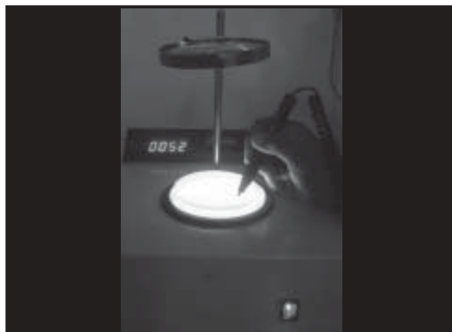
Figure 4: Colony counter for measuring the count of microorganisms
